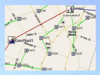
By right clicking the map, the software allows viewing one or multiple of the listed components. Regarding transmission lines, operators shall decide which lines to view through a transmission line form that permits displaying all lines, hiding all lines, showing specific links between generation plants and substations or specific lines with certain voltages.
